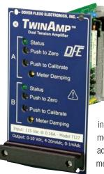
The TwinAmp is a rack-mount transducer interface for monitoring tension in any two tension—sensing zones simultaneously. Two independent, isolated amplifier circuits are included on one card saving you space and money. IEC/ANSI/IEEE type 2 plug-in card installs into standard size 3U 19
