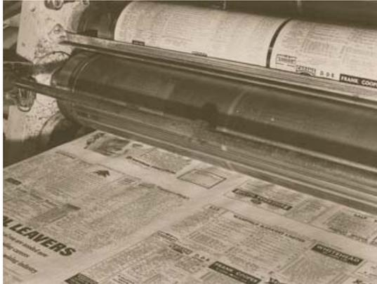
Identifying problems or deviations that cause running web breaks is not black magic. The solution starts with measuring the process variables that are critical to a successful print run on your press, including web tension.
