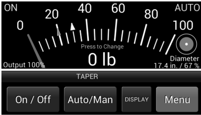
Figure 16 - TAPER SETPOINT ON METER
