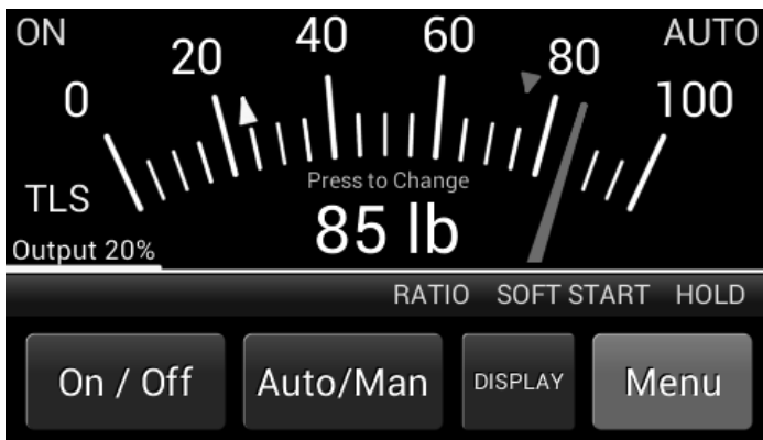
Figure 19 - TLS SETPOINT SHOWN
